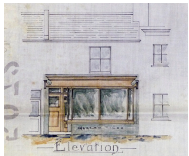
8 | Detail showing large Window Panes installed at No. 4, 1902. Image courtesy of East Sussex Record Office
