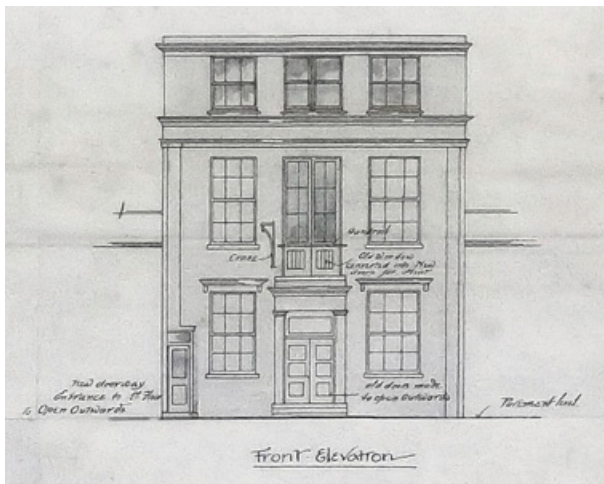
10 | Close-up of the Reason Manufacturing Company's Robert Street works, illustrating the main elevation with hoist. Image courtesy of East Sussex Record Office
